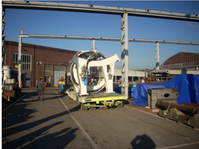
Photo3-2. Boring machine for tunneling
